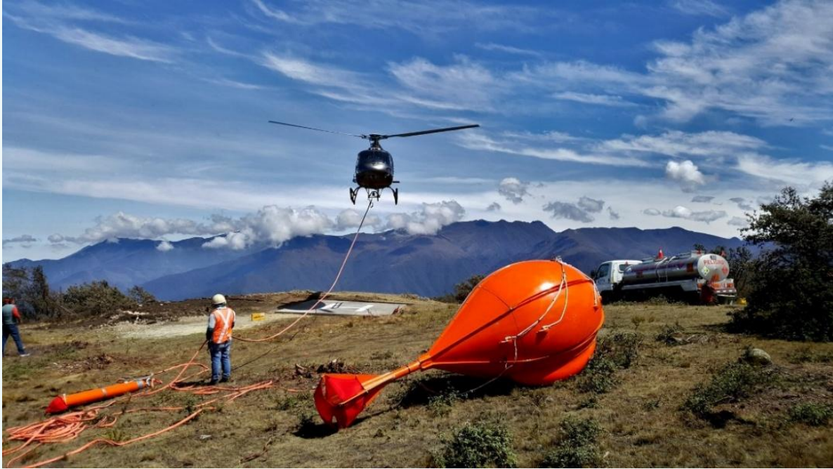
Figure 3. Example of a helicopter with a probe slung for airborne magnetics ( https://expertgeophysics.com/services/ )
