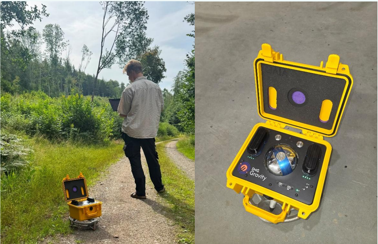
Figure 12. Gravity measurements along a gravel road at Hennes Bay (2026).
