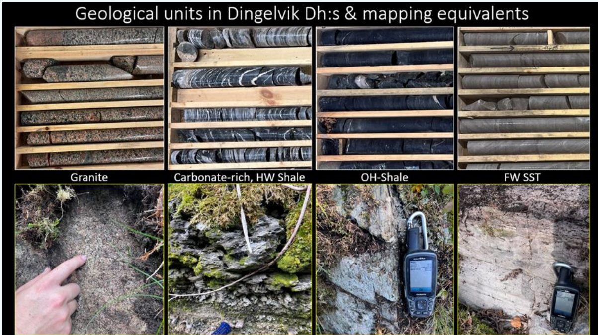
Figure 18: Visual correlation between field and drill core observations (REEM 2023)
